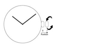
To set the time pull out the crown to position 1, turn to set your desired time and push back the crown to position 0.
