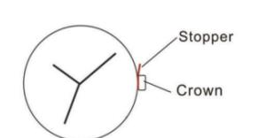
NOTICE: To make your watch working, remove the stopper located between the watch and the crown.
